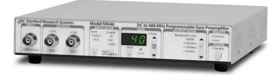
The SR446 is a single-channel, 400MHz bandwidth voltage preamplifier with 21 programmable gains from 1 to 100 (+0 dB to +40 dB with 2 dB steps). It also includes four programmable low-pass filters, with settings of full bandwidth, 200 MHz, 100 MHz and 20 MHz. There are two output channels which offer complimentary outputs (inverting and non-inverting) that can be used separately, or together as a differential output.
